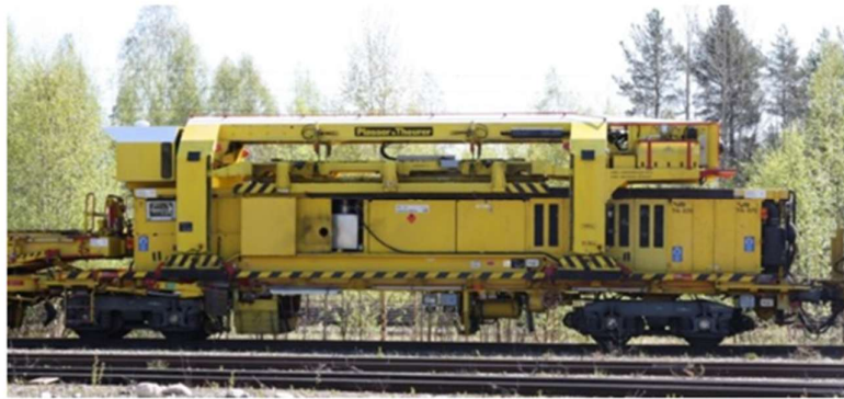
Example of transport together (portal crane on top of powerwagon)
